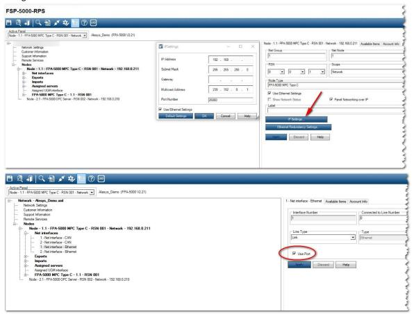
In the main node select **IP Settings** and configure IP address, Subnet Mask and other parameters as configured in the panel with the keypad.
