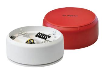
This device, if operated with an industrial, high-performance power source for bypassing the power supply ensures uninterruptible alarm signaling in line with VdS 3536, even if a stub line is broken or the bus system is permanently damaged (e.g. by fire). The power source is laser-welded, making it leak proof. The gold contacts allow the devices to be used in adverse environmental conditions. The control panel enables continuous and reliable monitoring of the power source.
