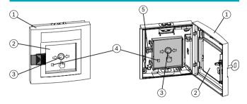
In the event of an alarm, the glass pane (2) is broken first, then the manual call point (3) is pressed hard. This activates the microswitch for alarm triggering and the indicator LED (4) blinks. A mechanism holds the pressed call point down.
