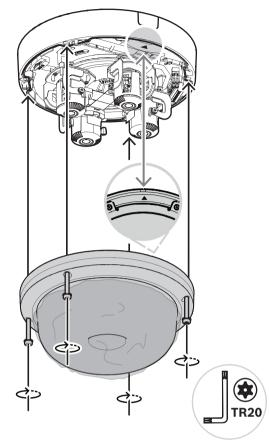
3. Remove the protective cover from the bubble.
