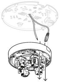
11. Fix the M20 rubber grommets in both cable inlets to make sure that the cable inlets are firmly closed.
