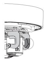
3. Do not tilt each of the four lenses any further than until the white dot on the edge of the lens holder meets the white triangle. If you tilt any further, you might see a partly blurry image. Use this position only in specific use cases or when you need the lens to fully zoom in.
