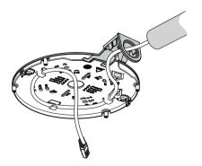
12. Install the conduit cover on the conduit plate with the bolt. Tighten the screw between 1.4 and 2 Nm (1 lbfft and 1.5 lbfft) with the TR20 Allen key.
