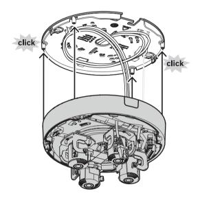
14. Tighten the 4 captive screws of the screw holes in the camera base between 4 and 7 Nm (3 and 5.2 lbfft).
