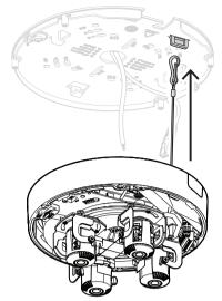
2. Put the RJ-45 punch-through aid on the network cable.
