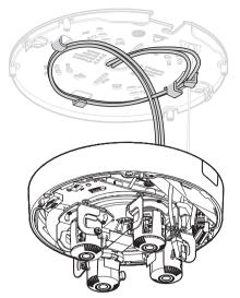
13. Position the camera base on the mounting plate, so that the screw holes of camera base and mounting plate match. Slightly press the camera base onto the mounting plate until you hear/feel a click. Make sure that the camera base is secured.
