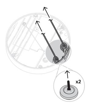
12. If required, do a loop with the cable on the hooks of the mounting plate.
