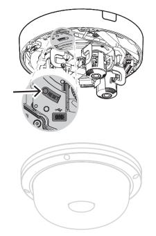
3. Re-attach the camera dome cover onto the camera base.
