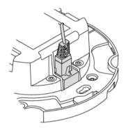
20. Pre-fix the camera module to the camera base with the spring hooks. Make sure that the arrow on the camera module points in the same direction as the arrow on the camera base.
