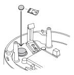
15. Connect the PoE cable to the camera module.
