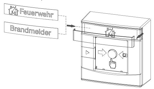
Figure 10: Mounting the door sign
