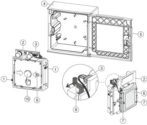
Figure 15: Replacing the battery pack
