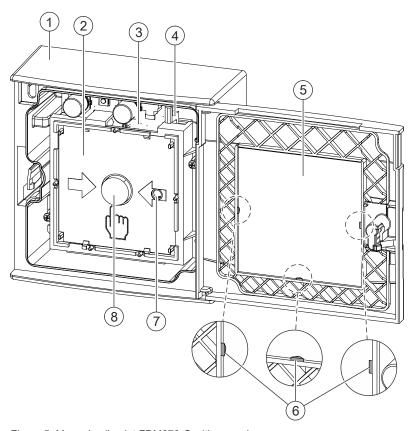
Figure 5: Manual call point FDM273-O with open door
