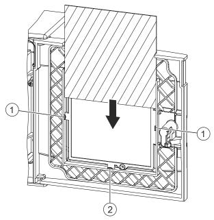
Figure 14: Replacing the glass insert
