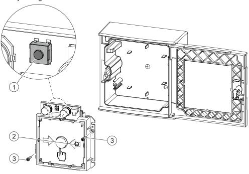
Figure 13: Establishing factory settings
