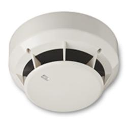
The device is UL 268 7th edition listed and is a reliable, high-quality multi-criteria Photoelectric Smoke Detector. It can be used in all open areas where Photoelectric Smoke Detectors are required. The newly developed multi-spectrum smoke categorization technology detects smoldering and flaming fires fueled by traditional materials and polyurethane while reducing nuisance alarms.
