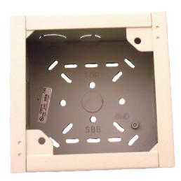
A white surface-mount back box measuring 14 cm  $(5.5 \text{ in.}) \times 14.2 \text{ cm} (5.6 \text{ in.}) \times 9.1 \text{ cm} (3.6 \text{ in.})$ . It has one 1.9 cm (0.75 in.) and one 1.3 cm (0.5 in.) knockout on each side.
