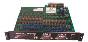
Modular design plug-in circuit board. Provides a shielded interface between the Conettix D6610 CPU Line Card and external connections to automation database computers and printers. Includes:
