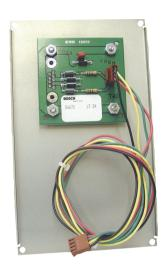
Creates a third serial port on the Conettix D6600 Communications Receiver/Gateway. Provides a DB9 male connector and transient protection.
