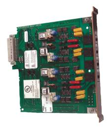
Modular design plug-in circuit board. Provides isolation and transient suppression to the Conettix D6641 Telephone Line Card. Provides four modular RJ11 jacks for telephone line connections.
