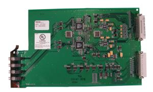
Line card with digital signal processor (DSP) technology. Answers and decodes signals from up to four telephone lines simultaneously. The Conettix D6600 Communications Receiver/Gateway will accept up to eight telephone line cards to create a total of 32 telephone lines. Needs one Connetix D6645 Telephone Line Terminator Card.
