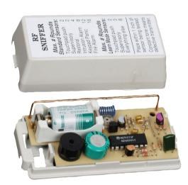
The Radio Frequency Sniffer tests sensors. It emits a series of beeps when RF transmission is detected. It emits a single constant tone when a transmitter is defective.
