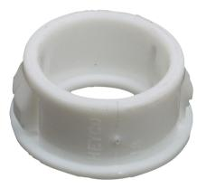
Used to adapt sensor magnet to a steel door by providing 0.6 cm (0.25 in.) plastic spacer around magnet. Provides extra thickness for proper alignment. Shipped in packages of 20.
