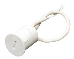
Recessed mount only in window frames. Connects externally to Learn Mode® Shock Sensors. Detects breaking glass up to 1.5 m (5 ft) radius from detector. Measurements: 2.2 cm x 3.5 cm x 1.0 cm (0.88 in. x 1.38 in. x 0.38 in.).
