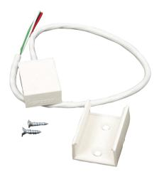
Surface mount on window frames. Connects externally to Learn Mode<sup>®</sup> Shock Sensors. Detects breaking glass up to 1.5 m (5 ft) radius from detector. Measurements: 2.2 cm x 3.5 cm x 1.0 cm (0.88 in. x 1.38 in. x 0.38 in.).
