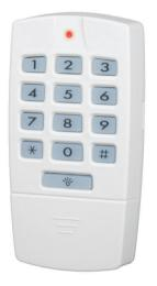
The RF3341 is a one-way wireless keypad transmitter with backlighting and key-press sounder, which allows the user to arm, or disarm, and send special codes anywhere within the range of the system receivers. The RF3341 is compatible with the RF3224 Receiver and with the RF3222 Receiver. The keypad can be wall mounted or portable. Control panel programming and control panel type determine which system functions are available from the wireless keypad.
