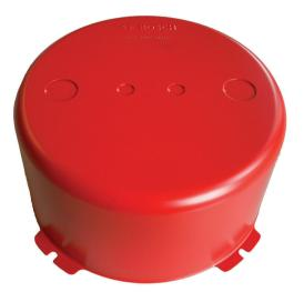
During a fire, the ceiling cavity in which loudspeakers are installed can allow flames to spread throughout a building. To prevent fire entering the cavity via the loudspeaker, the ceiling loudspeaker can be fitted with a steel fire dome. This optional fire dome is mounted on the loudspeaker assembly using four self-tapping screws supplied with the fire dome. The fire dome has knockout holes for two grommets (supplied) and two cable glands (PG 13).
