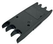
The network splitter allows the main network line to be split into branches. The branch lines are still supervised, but do not have the redundant cabling of the main network line. The network splitter has an option to connect a 48 VDC supply that can supply additional power if required. The network splitter can also function as a repeater to extend the cable another 50 meters with plastic fiber.
