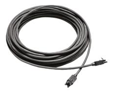
This is a special cable with 2 plastic fibers for data and audio communication and 2 copper cores for the power supply. The cable is supplied with the network connectors fitted. This cable can be used to connect the CCU to audio expanders.
