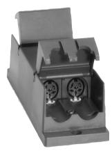
The Tap-Off Units create short-circuit proof tap-off points on the trunk line cabling. Each tap-off point allows for connection of up to five channel selector panels or one tabletop contribution unit such as Discussion unit, Concentus unit or Interpreter Desk. A Tap-Off Unit consists of two tap-off points. The Tap-Off Unit comes complete with cable restraining clamps and includes mounting holes for fixing purposes.
