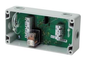
The Universal Connection Relay (UAR) is controlled by a security system and handles the triggering of additional equipment on monitored control lines. The UAR can be, depending on the connection to the security system, equipped with a 12 V relay or a 24 V relay.
