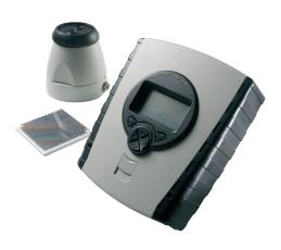
The FRAY5000-EN Linear Smoke Detector covers distances between 8 m and 100 m. A reflective prism allows for the accurate detection of smoke particles within the given distance range.
