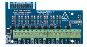
The CM707B Plug On Zone Expander is designed to complement the CM705B Universal Zone Expander. It can be added via the expansion port on the CM705B Universal Expander to provide an additional 8 hard wired zone inputs, bringing the CM705B to 16 hard wired zone inputs for Alarm + Tamper, 4 state monitoring or Single EOL configurations.
