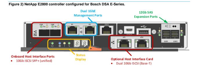
**Note:** Although the NetApp E-Series E2800 supports multiple host interface options, the Bosch VMS integrated DSA E2800 solution supports one configuration, shown in Figure 2.
