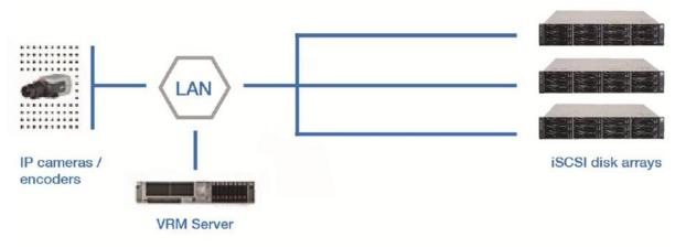
Figure 8) Concept drawing of basic Bosch VRM solution.
