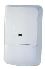
This detector is used for monitoring rooms for unauthorized entry.
