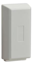
The DS7460i Dual-zone Input Module works with compatible multiplex systems, uses two multiplex zone addresses, and monitors up to two separate zones. It is DIP switch programmable and provides two supervised input zones to connect conventional normally-open (NO) or normally-closed (NC) contacts.
