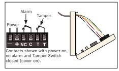
Figure 4.1: Wiring the detector
