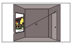
Figure 3.1: Opposite wall mounting using door contact
