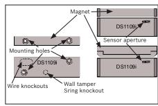
Figure 8.1: Mounting the Detector
