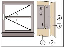
Figure 3.4: Single window coverage using the magnetic contact
