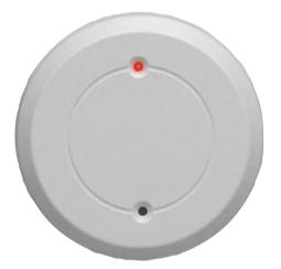
The DS1100i Detector Series uses microprocessorbased sound analysis technology (SAT) to listen for the specific frequencies associated with breaking glass. The DS1101i, DS1101i-BEL, DS1101i-CHI, and DS1101i-FRA can be used to detect breakage of plate, tempered, laminated and wired glass types. A built-in environmental test feature alerts the installer to false alarm hazards in harsh environments. The round detectors mount on the ceiling or walls.
