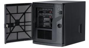
DIVAR IP all-in-one 4000 is an affordable and easy to use all-in-one recording, viewing, and management solution for network surveillance systems of up to 32 channels (with 8 channels pre-licensed).
