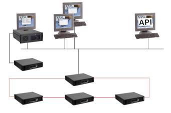
DCN-SWAPI-E is deployed as Microsoft.Net components to be used by 3rd party applications to control, modify, add, remove and update a subset of the DCN-SW-E configuration data to prepare meetings. It also includes a subset of the DCN-SW-E control functionality to control meetings.
