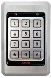
The D8229 Access Keypad sends output in a Wiegand 26-bit format. Enter a personal identification number (PIN) to obtain access. There are keys for numbers 0 through 9, for the number symbol (#), and for the asterisk symbol (\*). Each time you press a key, one of the light emitting diode (LED) indicators emits a red light and an annunciator emits a beep.
