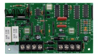
The D8125 Addressable Expansion Module works with the D9127U or D9127T POPIT Modules to provide multiplex technology that combines zone or point supervision with individual device addressing on one pair of wires. Use the D8125 to provide expansion beyond the standard number of control panel zones, up to a total of 238 points. Each D8125 module can fully supervise 119 D9127U or D9127T POPIT Modules.
