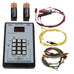
Required for programming the multiplex bus points on D9412G, D7412G, and D7212G Control Panels. Also use it to program and read information from a D8125 MUX.
