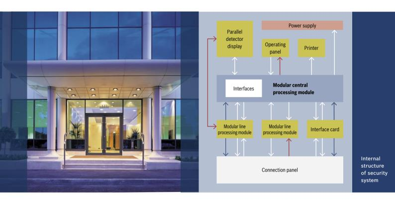
Security systems were previously put together using many individual components. The Universal Intrusion and Fire Alarm Panel 2000 Series LSN now integrates all necessary security components into a single system. A central location controls the functions and measures for fire and intruder surveillance.
