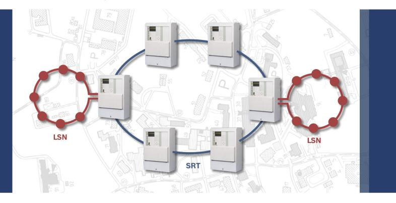
With SRT system ring technology you can, according to your individual needs, arrange up to six control units in a centralized or decentralized configuration.
