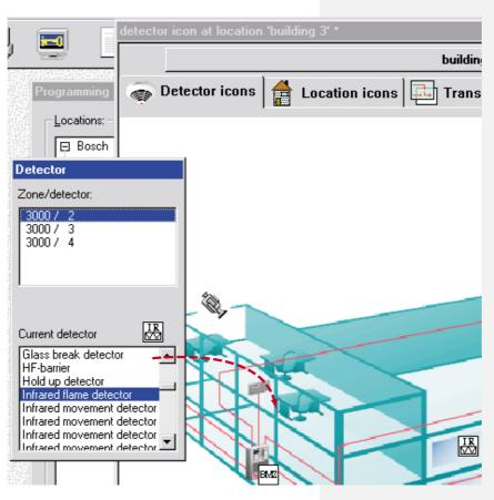
Positioning the detector using Drag & Drop
