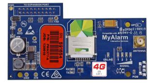
The CM748B 4G LTE CAT 1 radio module allows you to interface compatible security control panels to the CAT 1 cellular network providing a high reliability primary or backup reporting path.
