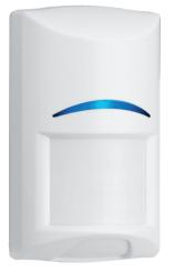
The Blue Line Gen2 TriTech Motion Detectors (ISC-BDL2) use a combination of passive infrared (PIR) and microwave Doppler radar detection with advanced signal processing. The pet-friendly (-WP) models generate alarms for human intruders without generating false alarms for pets. These small unobtrusive detectors are simple to install and do not need field adjustments.
