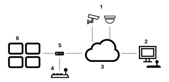
Figure 6.2: Scenario 2: Bosch IntuiKey keyboard connected to a decoder
