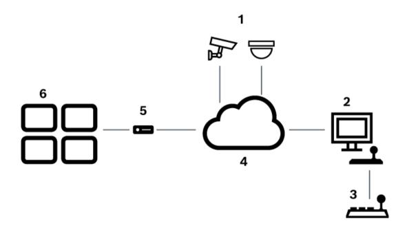
Figure 6.1: Scenario 1: Bosch IntuiKey keyboard connected to a Bosch Video Management System workstation
