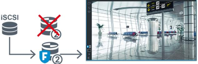
When the Secondary VRM and the optional Secondary Failover VRM are both not connected, the encoder provides playback. Close the Image pane and drag the camera again to an Image pane:
