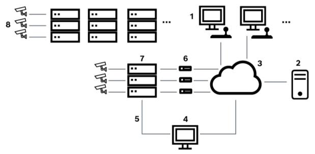
Figure 6.5: Bosch Allegiant system extended with Satellite switches
