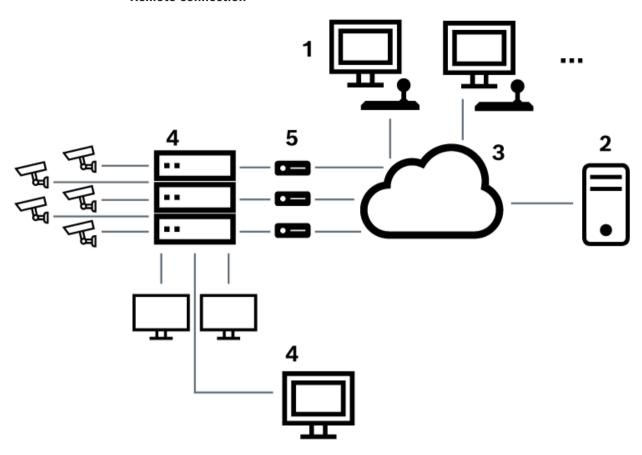
Figure 6.4: Bosch Video Management System remote connection to a Bosch Allegiant matrix switch
