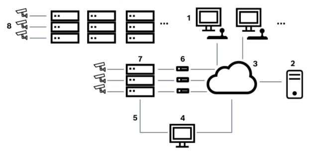
Figure 5.5: Bosch Allegiant system extended with Satellite switches
