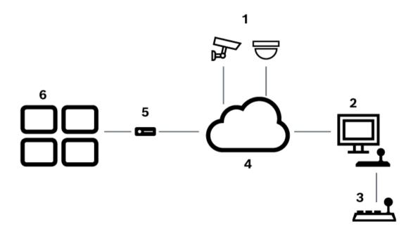
Figure 5.1: Scenario 1: Bosch IntuiKey keyboard connected to a Bosch Video Management System workstation
