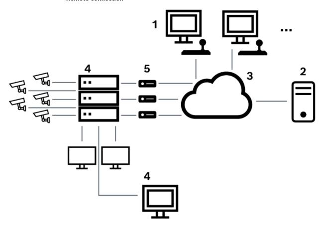
Figure 5.4: Bosch Video Management System remote connection to a Bosch Allegiant matrix switch
