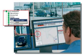
The **Operator Alarm** feature allows an operator to trigger an alarm manually from the location tree, for example, if informed by telephone of a dangerous situation. Such manual alarms are processed in the same way as those triggered by a detector: that is, the associated documents are displayed and all steps taken are recorded in the event log for thorough postevent investigation.
