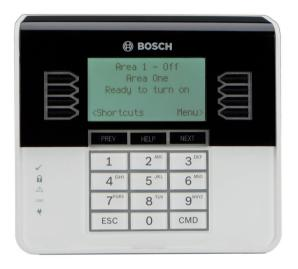
The B930 ATM Style Alphanumeric Keypad (SDI2) is a SDI2 bus compatible device. Each keypad has user adjustable options such as volume and display brightness. The B930 shows five-line system messages for all areas.
