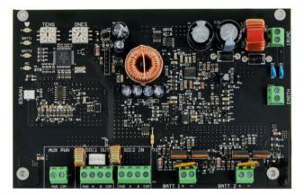
The B520 Auxiliary Power Supply Module is an auxiliary power supply expansion device that connects to compatible control panels through the SDI2 bus. This module is supervised and communicates all status changes to the control panel.
