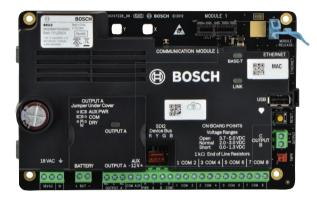
The B3512 Control Panel integrates intrusion and residential fire, providing one simple user interface for both systems. The B3512 provides up to 16 individually identified points in a single area. The control panel communicates via the built-in Ethernet port or via compatible plug-in modules that can send events over the public switched telephone network (PSTN) or over cellular network communications.
