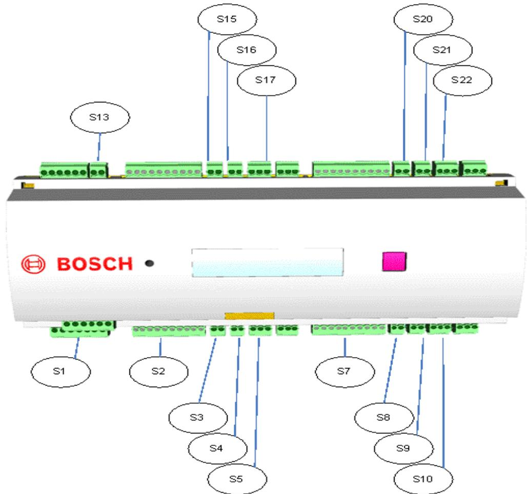
**Figure 3.5** The AMC2 connections used in the 4-room surgery example.
