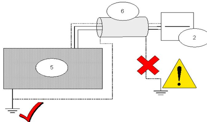
**Figure 3.3** Avoiding a ground loop
