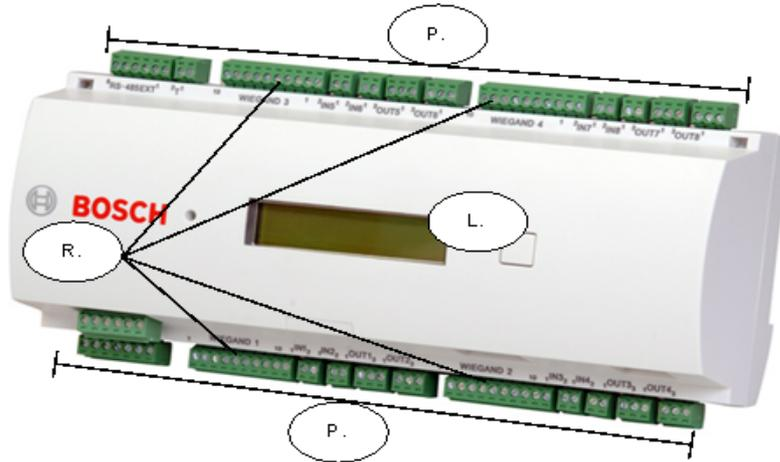
**Figure 3.4** An AMC2 access controller
