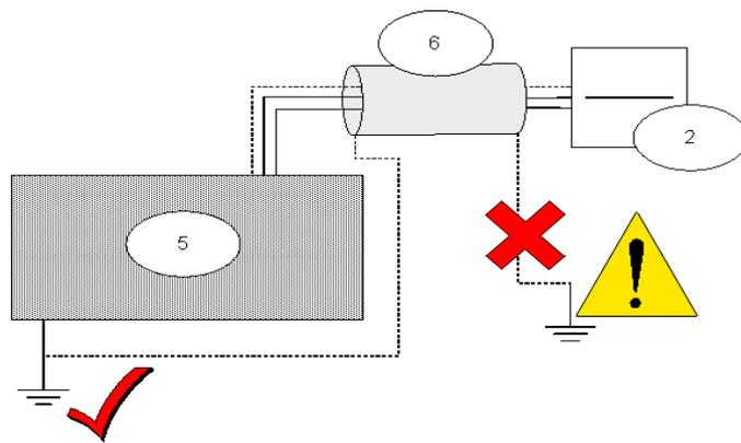
Figure 4.3 Avoiding a ground loop
