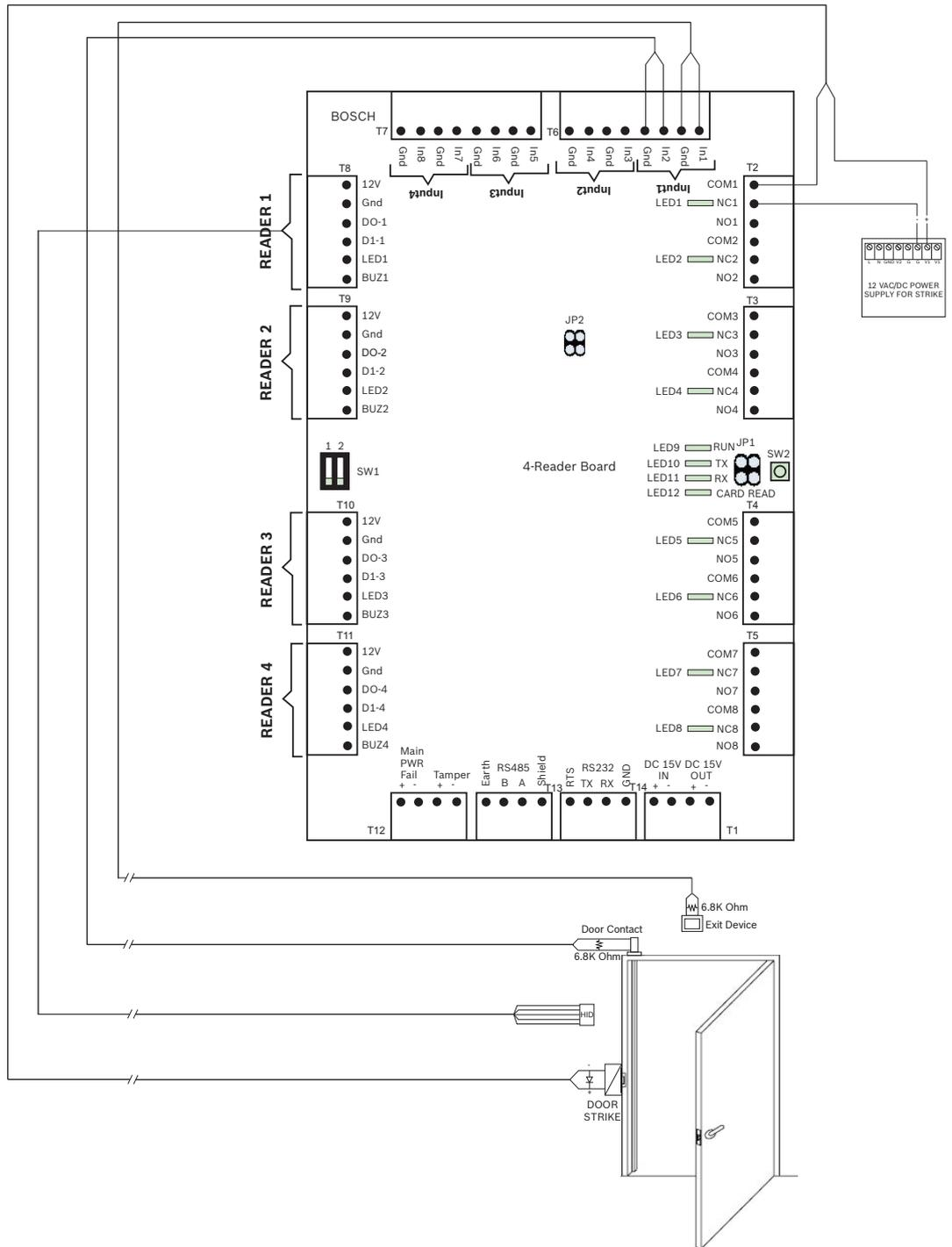
**Figure 4.5** The AEC2.1 connections showing one of the door connections.
