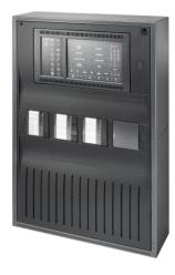
The fire panel allows mixed operation of analog addressable and conventional technology. It supports connecting periphery in either stub or loop topologies. Analog addressable fire detectors, manual call points, signaling devices, inputs and outputs are identified and managed by the fire panel as single elements. As required by the building structure the peripherals are grouped software wise in logical zones.
