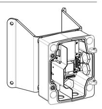
Figure 6.2: Power Supply Wall, Mast (Pole), and Corner Mounts
