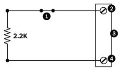
Figure 15.47: N.C.S. - Normally Closed Supervised Connections
