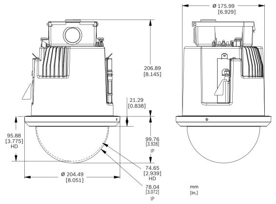
Figure 9.29: AUTODOME 7000 Dimensions - In-ceiling
