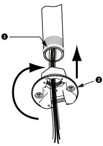
Figure 8.23: Attach Dome Cap
