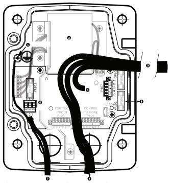
Figure 8.18: Power Supply Box Connections
