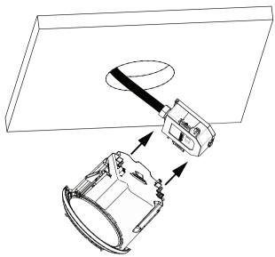
Figure 9.38: Attach Housing to Interface Box
