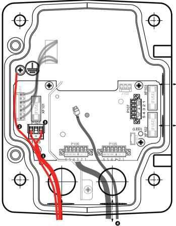
Figure 7.8: VG4-PA0 Power Supply Box
