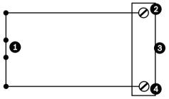
Figure 15.49: N.C. Normally Closed Non-supervised Connections
