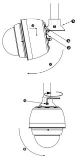
Figure 8.28: Pendant to Roof / Pipe Mount Attachment
