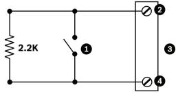
Figure 15.46: N.O.S. - Normally Open Supervised Connections
