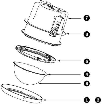
Figure 9.37: In-ceiling (IP54 Rating) Installation Diagram
