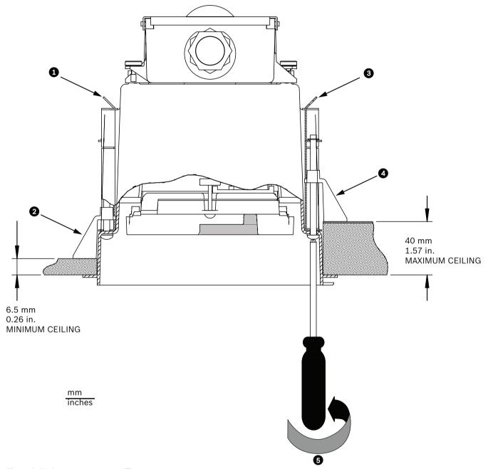
Figure 9.40: Secure camera to ceiling
