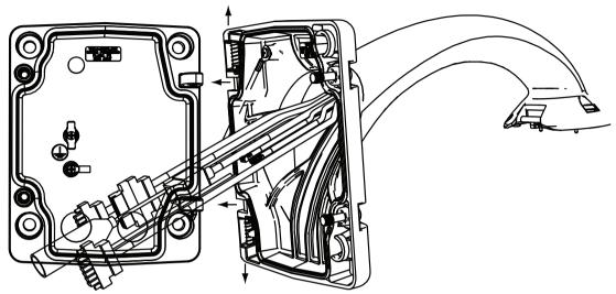
Figure 7.11: Connect Pendant Arm to Mounting Plate
