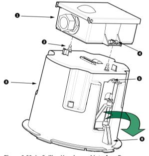
Figure 9.39: In-Ceiling Housing and Interface Box
