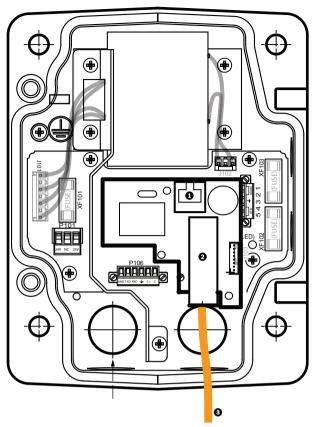
Figure 8.17: Fiber Optic Ethernet Module installed
