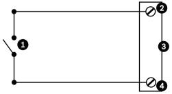
Figure 15.48: N.O. - Normally Open Non-supervised Connections
