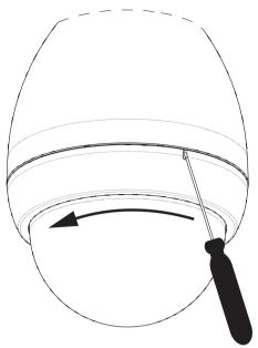
Figure 10.42: Pendant Bubble Release Opening
