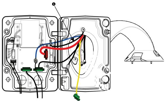
Figure 7.10: Pendant Arm connections to Power Supply Box
