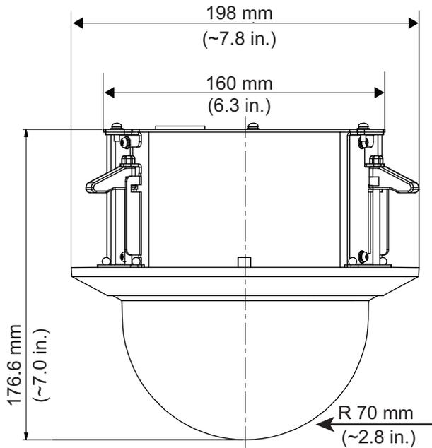
Fig. 6: In-ceiling model
