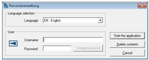
After entering a username and password, the button **Change Password** becomes active. After 3 wrong entries a time delay before the next logon will be the consequence. This applies for the buttons "Start the Application" and "Change Password".
