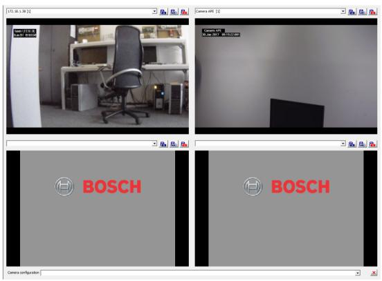
In the video panel it is possible to select up to four cameras from different entrances. The following functions are available for each display window.
