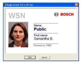
The **Print** button begins the print process by invoking a dialog to choose a printer. If a default printer has been defined in Configurator then printing proceeds immediately.
