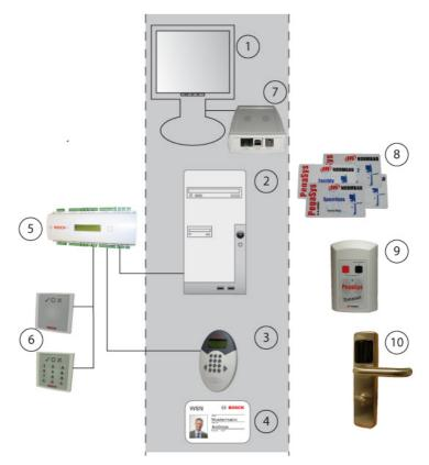
When the locking system is integrated into the Access PE access control system, certain components are used by both systems. The gray area in the diagram above contains the system components that are used by both the access control system and the locking system. The items on the left are purely access control installations and the items on the right belong only to the locking system.
